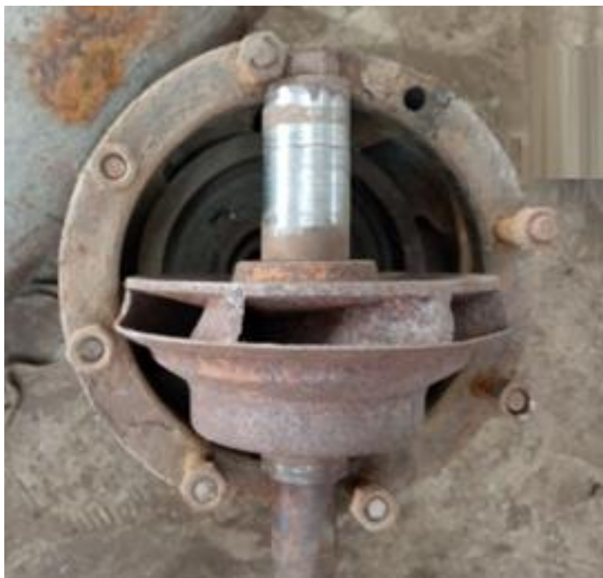
Figure 4. Experimental testing of ECW submersible pumps on dedicated test benches during performance evaluation: Internal view of impeller.
