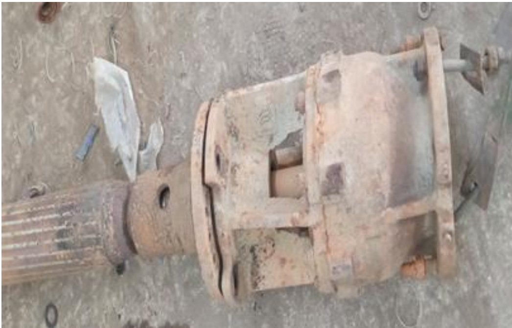
Figure 5. Experimental testing of ECW submersible pumps on dedicated test benches during performance evaluation: External view of pump.
